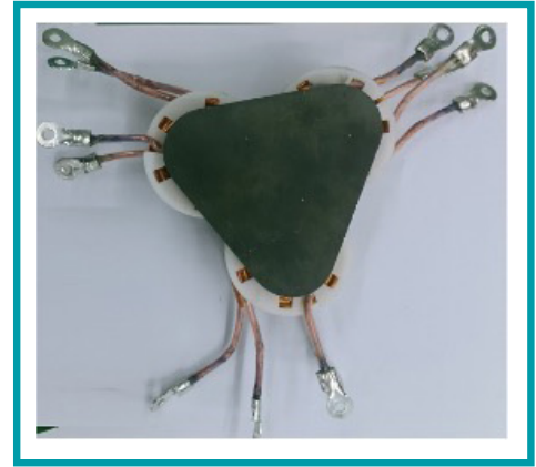
Fig. 13 22kW CLLC Transformer prototype sample
