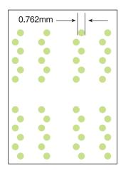
Figure 4. BGA device stencil example
