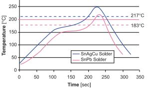
Figure 6. Typical solder reflow profile
