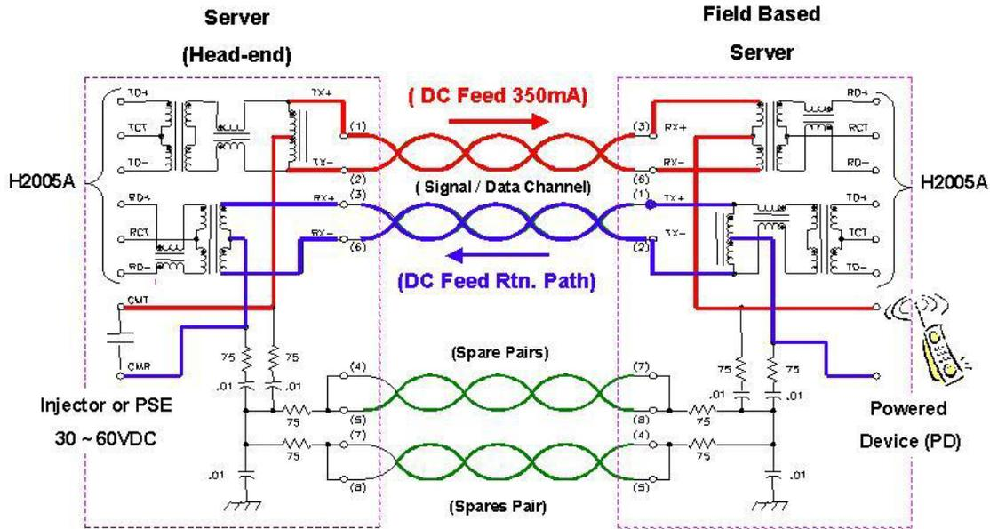
**Figure 2 Power-over-Ethernet Example**
