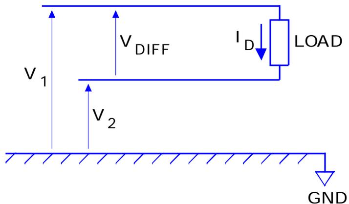
In a cable based transmission system the Differential Mode signal is the "wanted" signal that carries information. All Physical Layer (PHY) transceivers for LAN and Telecom applications are differential mode devices
