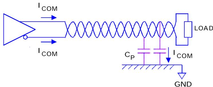
parasitic capacitance  $C_P$ . In this case, the currents generate magnetic fields with equal magnitude and polarity, which do not cancel each other out. The common mode current is able to generate an electromagnetic field outside the spiral wound pair, which acts just like an antenna.
