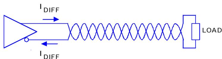
For pure differential mode signals, the currents in each of the wires in a pair travel in opposite directions. If the pair is uniformly wound these opposing currents produce equal and opposite polarized magnetic fields that cancel each other out.
