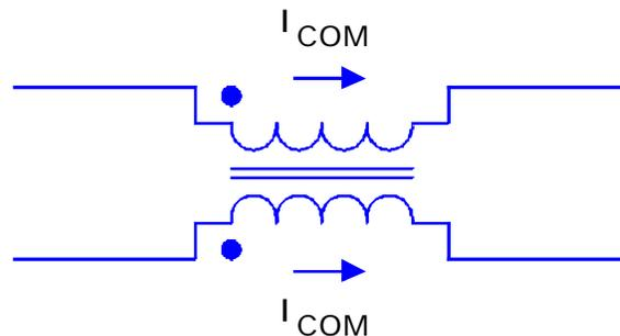
presenting a high impedance to the common mode signal, which passes through the choke heavily attenuated. The actual attenuation (or common mode rejection) depends on the relative magnitudes of the choke impedance and the load impedance.
