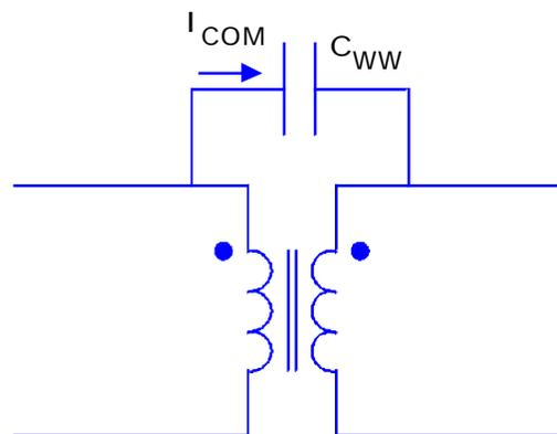
and the presence of a dielectric between the windings. The size of this Interwinding capacitance can be reduced by increasing the separation between the windings, and by using a low permittivity material to fill the space between the windings.
