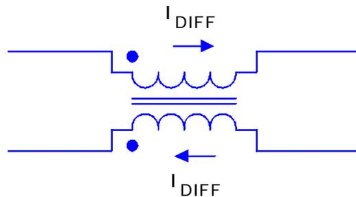
presenting zero impedance to the differential mode signal, which passes through the choke unattenuated.
