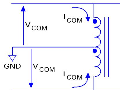
magnetic fields to be generated which cancel each other out. The effect is that the device presents zero impedance to common mode signals, shorting them directly to ground potential.
