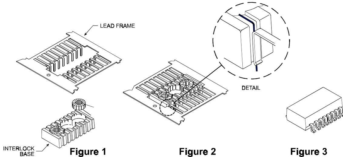
The InterLock Base allows for physical isolation of the coils from the encapsulation, while at the same time providing a mechanism for high density integration of multiple magnetic components within a single SMT package. See **Figure 4** below.
